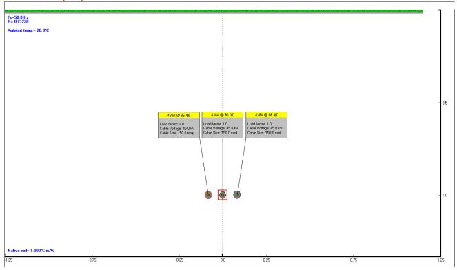
Cables in earth → Single-point Ampacity 417A
