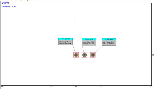
Cables in air  $\rightarrow$  Single-point shaded Ampacity 467A
